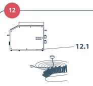
With a nylon brush, clean the fan guard and air intake grille (12.1) on the underside of the unit. All debris should be removed so that air flow is not impeded.
