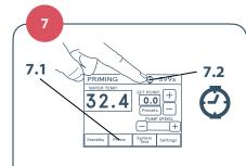
Run the MCH through five (5) standard priming cycles (**7.1**), or one extended priming cycle (**7.2**), to fully mix and circulate the cleaning chemical (10 minutes total).
