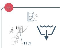
Turn off the mains power switch, and drain the system completely (11.1). If necessary, repeat the flushing sequence until all cleaning chemical is removed from the system.
