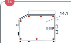
Internal tubing inspection: Instruct a qualified serviced personnel to unplug the unit and remove the side panel (14.1) from the device. Visually inspect the clear internal tubing. If the tubing does not appear clouded or discolored, reattach the side panel.
