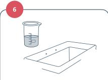
Add the selected cleaning chemical\* to the cold water tank at the manufacturer's recommended rates. Once primed, and with six inches of water in the tank, the MCH-1000(m) contains approximately 1 gal (4L) of water.
