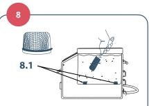
Scrub the cold water tank and outlet screens with a nylon brush. It is imperative that the tank and screens (8.1) be thoroughly cleaned to ensure disinfection. The screens may be unscrewed and removed to assist in cleaning. Be sure to replace the screens before operating the MCH.
