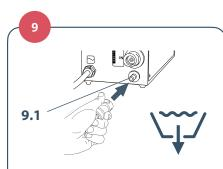
Attach the tank drain (9.1) connector and drain the unit completely. With the drain connector attached, flush the unit with sterile or 0.22-micron filtered water.
