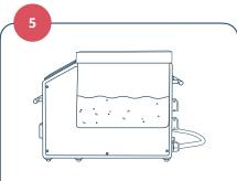
After priming, ensure the water level in the ice tank does not drop below four inches by adding sterile or 0.22-micron filtered water as necessary.
