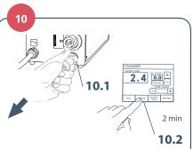
Disconnect the drain connector (10.1) and fill the cold water tank to maximum level with sterile or 0.22-micron filtered water. Run the MCH through a priming cycle (10.2) to flush residual cleaning chemical from the system.
