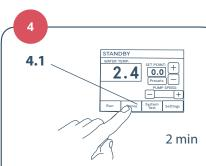
Touch the button (4.1) to initiate the priming sequence. The pump should turn on at full speed, and the valve should switch from COOLING to RECIRC approximately every ten seconds (check for ten-second bursts of water flow in the water tank).
