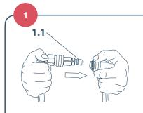
Attach the hoses with a loopback connector, MCH-10LBC (**1.1**), and put approximately six inches of sterile or 0.22-micron filtered water in the water tank.
