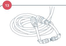
Inspect all plastic tubing on the hose kits. Any tubing that is clouded and/or has lost its flexibility should be replaced. To ensure proper function, exterior tubing must be replaced every 2 years regardless of condition. Replacement involves the detachment of the current hose and attachment of new hoses as outlined in the Maintenance section of the operator's manual.
