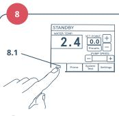
Press the Run button (8.1) to start the flow of temperaturecontrolled water
