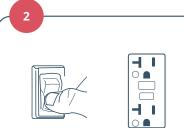
With the front panel mains power switch turned off, plug the power connector into a dedicated "hospital grade" AC power outlet. The outlet should match the voltage, frequency and capacity listed on the MCH nameplate.
