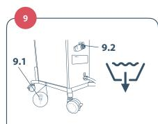
Open the system (9.1) and tank drain (9.2) valves and drain the unit completely. With the drain valves open, flush the unit with sterile or 0.22-micron filtered water.
