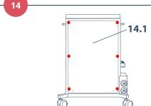
Internal tubing inspection: Instruct a qualified serviced personnel to unplug the unit and remove the side panel (14.1) from the device. Visually inspect the clear internal tubing. If the tubing does not appear clouded or discolored, reattach the side panel.
