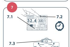
Run the MCH through five (5) standard priming cycles (7.1), or one extended priming cycle (7.2), to fully mix and circulate the cleaning chemical (10 minutes total). At some point during this step, set the recirculation valve to INTERNAL (7.3) for at least 10-15 seconds, to ensure that disinfectant reaches all sections of the internal plumbing.
