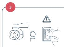
Turn on the mains power switch for the MCH. Ensure that the unit runs through a successful system
