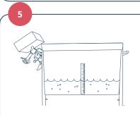
After priming, ensure the water level in the ice tank does not drop below four inches by adding sterile or 0.22-micron filtered water as necessary.
