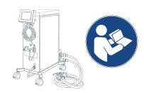
Perform the procedure listed under After Every Use in the Operator's Manual. The system can now be returned to use or stored. Always store the system drained and dry.
