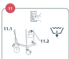
Turn off the mains power switch, and drain the system completely (**11.1** and **11.2**). If necessary, repeat the flushing sequence until all cleaning chemical is removed from the system.
