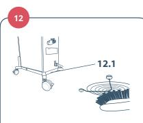
With a nylon brush, clean the fan guard and air intake grille (12.1) on the underside of the unit. All debris should be removed so that air flow is not impeded.
