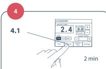
Touch the button (**4.1**) to initiate the priming sequence. The pump should turn on at full speed, and the valve should switch from COOLING to RECIRC approximately every ten seconds (check for ten-second bursts of water flow in the water tank).
