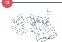
Inspect all plastic tubing on the hose kits. Any tubing that is clouded and/or has lost its flexibility should be replaced. To ensure proper function, exterior tubing must be replaced every 2 years regardless of condition. Replacement involves the detachment of the current hose and attachment of new hoses as outlined in the Maintenance section of the operator's manual.
