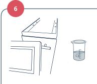
Add the selected cleaning chemical\* to the cold water tank at the manufacturer's recommended rates. Once primed, and with six inches of water in the tank, the MCH-1000(i) contains approximately three gallons (12 liters) of water.
