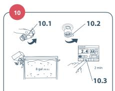
Close the drain valves (10.1 and **10.2**) and fill the cold water tank to maximum level with sterile or 0.22-micron filtered water. Run the MCH through a priming cycle (10.3) to flush residual cleaning chemical from the system.
