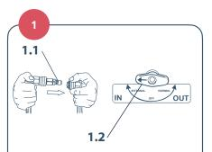
Attach the hoses with a loopback connector, MCH-10LBC (1.1) (or set the recirculation valve to INTERNAL (1.2), and put approximately six inches of sterile or 0.22 micron filtered water in the
