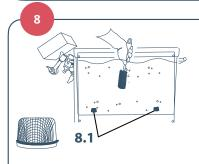
Scrub the cold water tank and outlet screens with a nylon brush. It is imperative that the tank and screens (8.1) be thoroughly cleaned to ensure disinfection. The screens may be unscrewed and removed to assist in cleaning. Be sure to replace the screens before operating the MCH.
