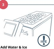
With Refrigeration Module: fill the cold water tank with approximately 8 gallons (30L) of sterile or 0.22-micron filtered water.
