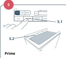
Press the **Prime** button (**5.1**) to clear the air from the water circuit. Allow the prime cycle to run for 2 min. (120s). Once the prime cycle is complete, top off the cold water tank with sterile or 0.22-micron filtered water so that water reaches the top edge of the inner shelf (**5.2**) of the tank.
