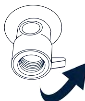
System Drain Closed
